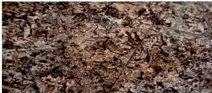
**FIGURE-33 OPTICAL MICROGRAPH OF BRASS EXPOSED FOR 15 DAYS
