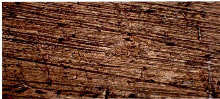
**FIGURE-34 OPTICAL MICROGRAPH OF BRASS EXPOSED FOR 15 DAYS
