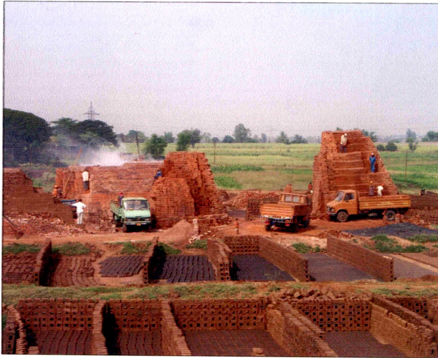
a) Brick kiln operation at all stages, raw material, brick drying, brick firing and loading for transport. Note the location of kiln in agricultural field (Shiroli Naka Site)
