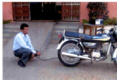
d) Testing of two wheeler exhaust with AEA
