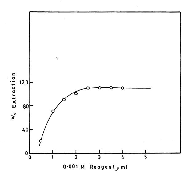
Fig. 1 - EFFECT OF REAGENT CONCENTRATION . Au (III) = 300 Jug
