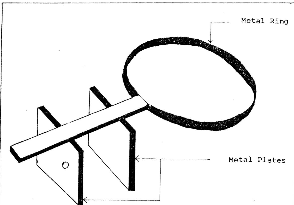
Fig.3.2. Reaction vessel stand.
