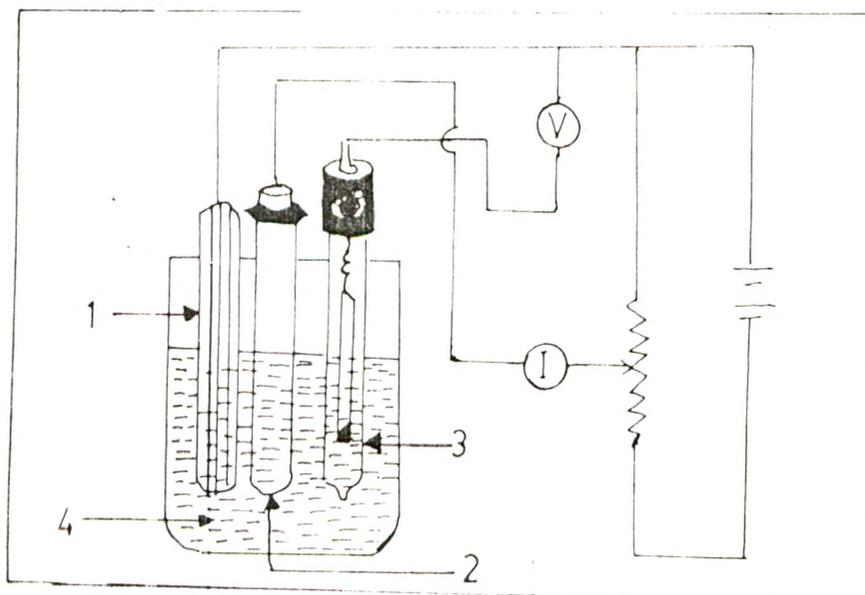
Fig.3.8 Experimental arrangement for electrical characterisation of a PEC cell:
