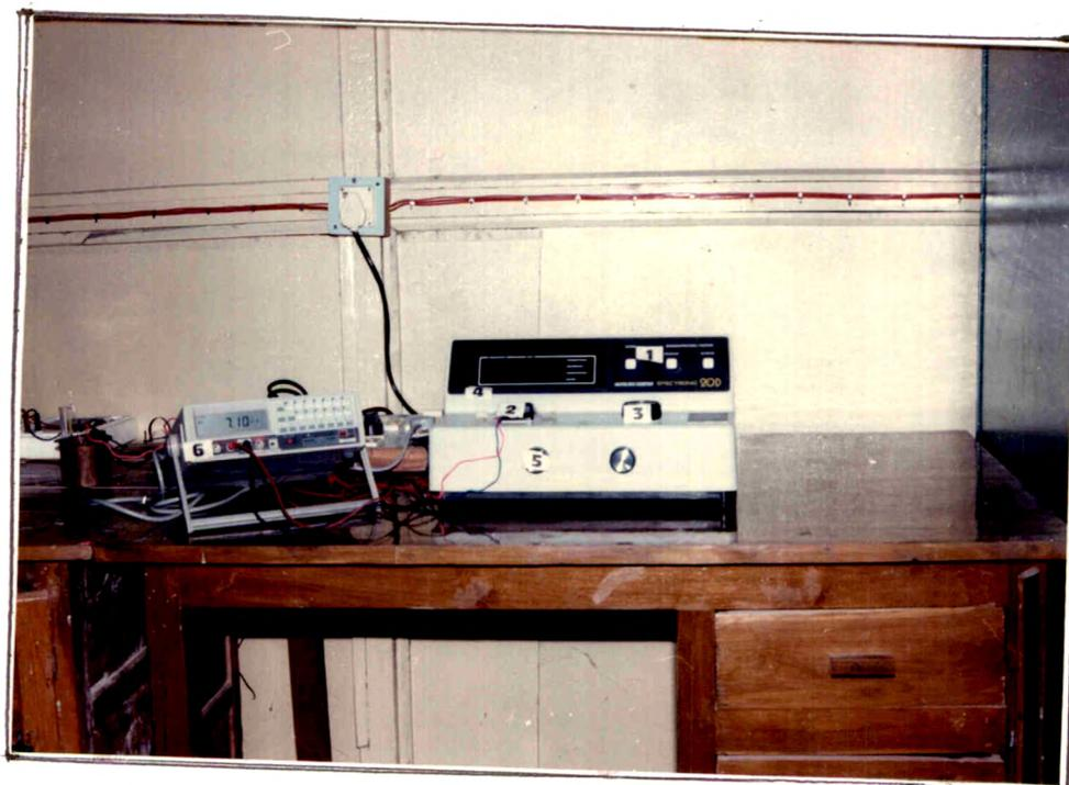
Fig. 3.9 Photograph of the experimental setup for spectral response of a PEC cell:
