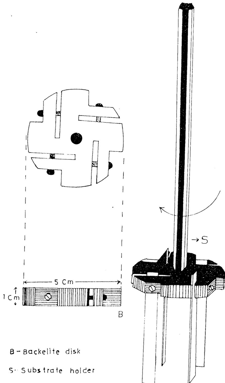
Fig-3-3 Design of the substrate holder
