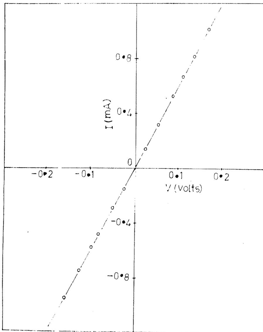
Fig.3.7. Nature of contact between  $\text{Bi}_2\text{S}_3$  and Stainless Steel substrates.
