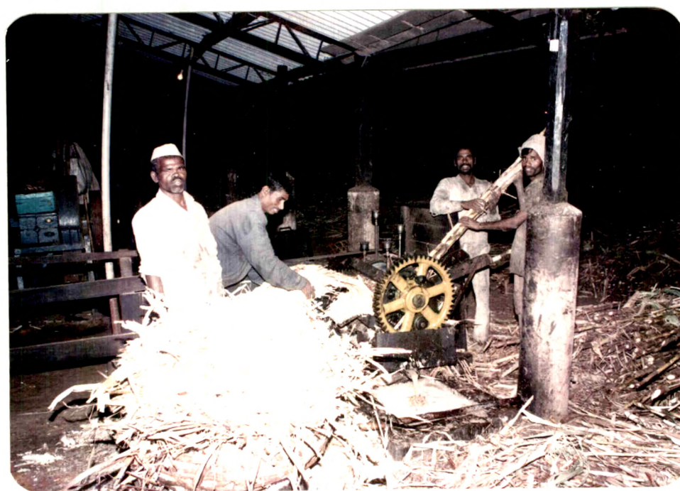
4. A PICTORAL VIEW OF Sugarcane Crushing (Extraction of Juice) (photo No.4.4)
