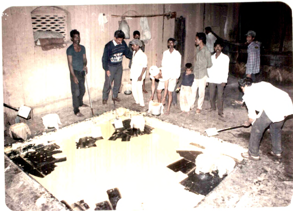
10. A PICTORAL VIEW OF Filling of Jaggery in Moulds (Photo No.4.10)
