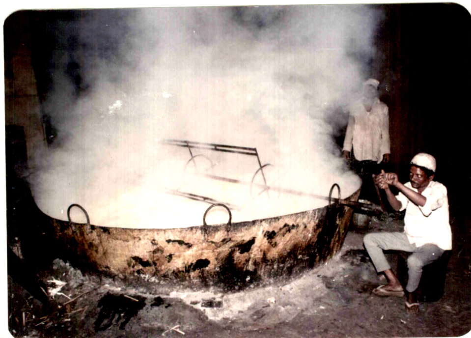
6. A PICTORAL VIEW OF Removal of Scum (Photo No. 4.6)
