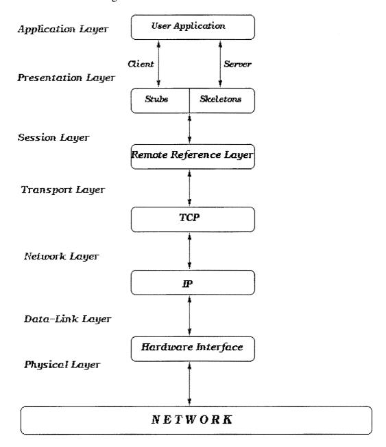
The User's application is at the top layer, it uses a data representation scheme to transparently communicate with remote objects, possibly on other Java Virtual Machine hosts.
