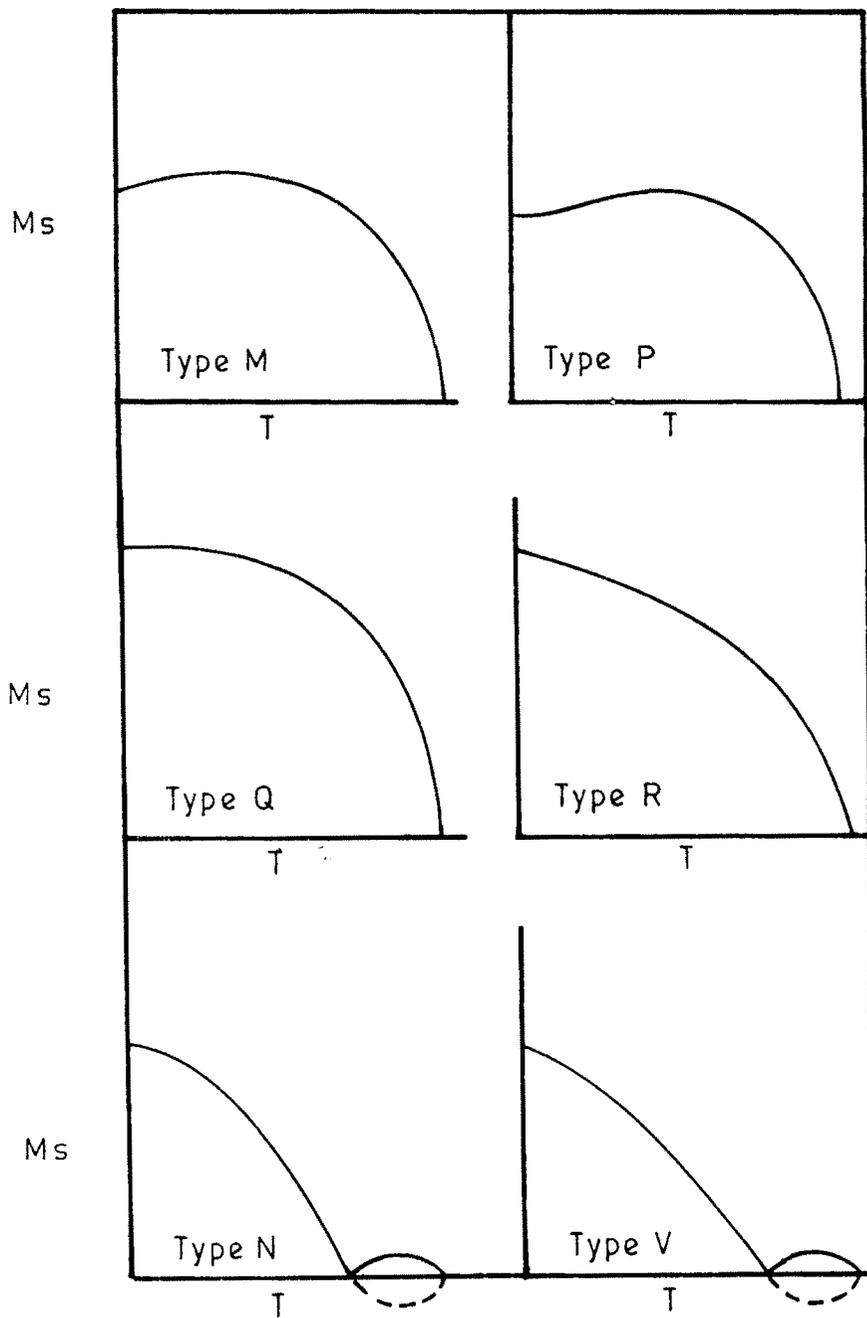
Fig.1-7  $M_s$  vs  $T$  Curves for ferrimagnetic substances predicted by Neel's Theory.
