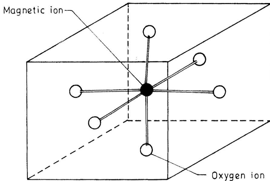
Fig. 1.3 The magnetic ion is said to occupy an "Octahedral lattice site" where it is surrounded by six near-neighbour Oxygen ions.
