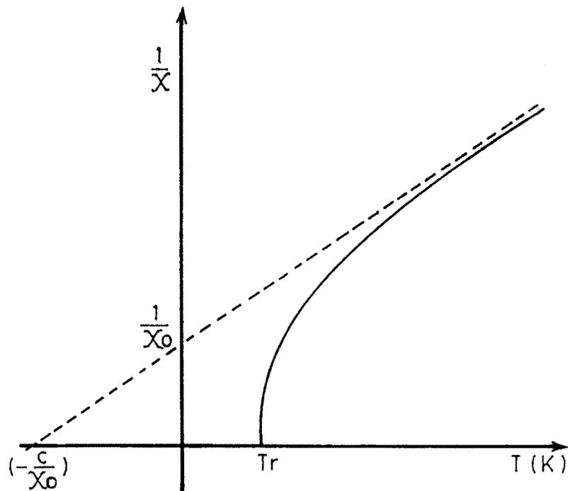
Fig. 1-5: Predicted susceptibility curve of a ferroelectric material above the curve point.
