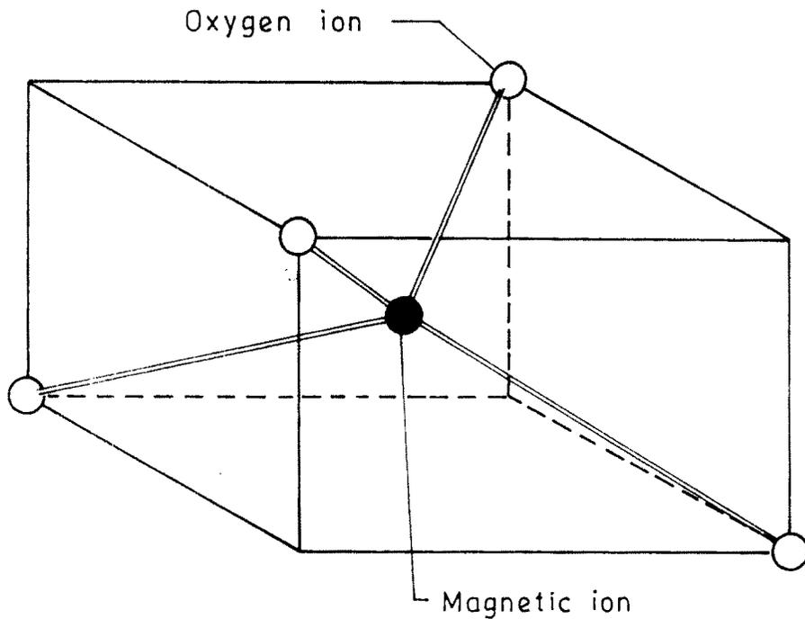
Fig. 1.2 : The magnetic ion occupies a "Tetrahedral lattice site" where it is surrounded by four near-neighbour Oxygen ions.
