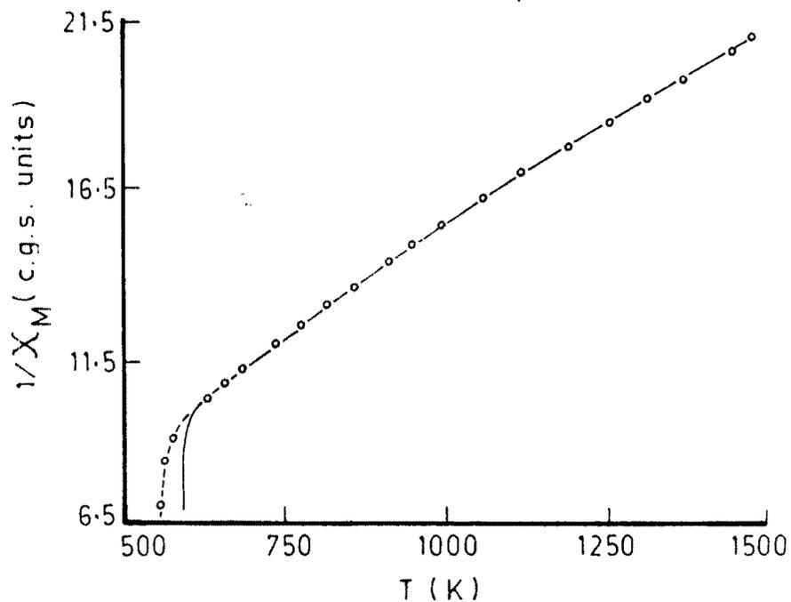
Fig. 1-6: Experimental susceptibility/ temperature curve for gadolinium-iron garnet.
