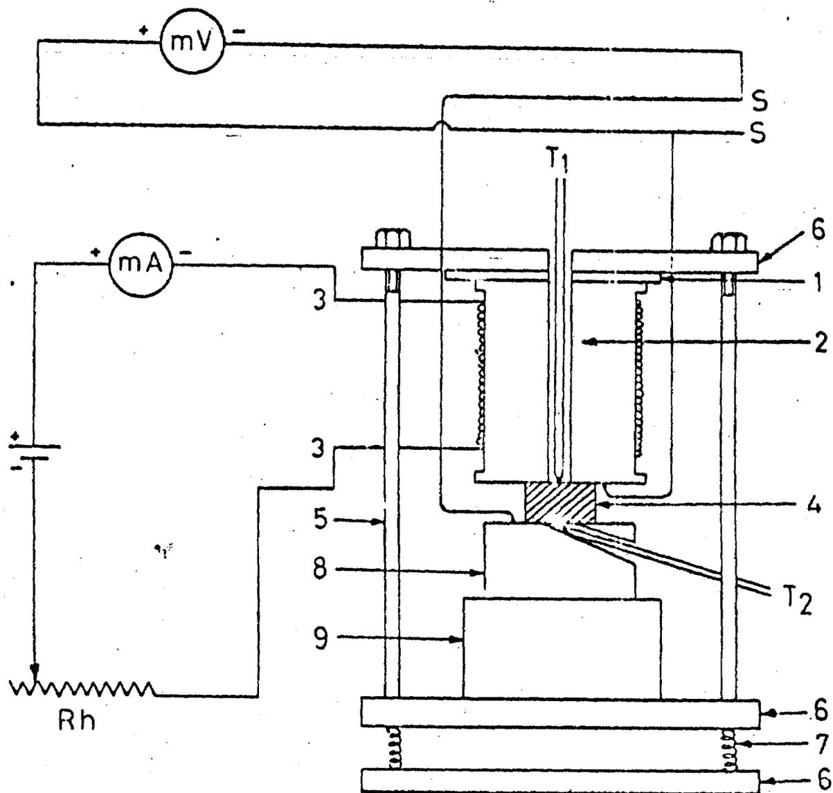
[1-Mion sheet; 2,8-Hard metal electrodes,3-Sub heater leads,4-Sample pellet,5-Metal rod;6-Metal plates;7-Spring,9-Metal block;T<sub>1</sub> T<sub>2</sub> - Thermocouples;S- Silver wires welded at Ag electrodes.]
