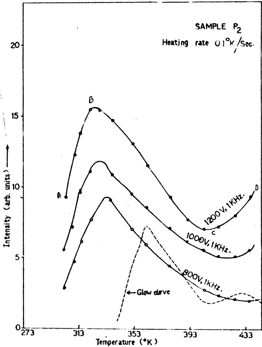
FIG. 4.1 PLOTS OF INTENSITY V/S TEMPERATURE AT DIFFERENT VOLTAGES.
