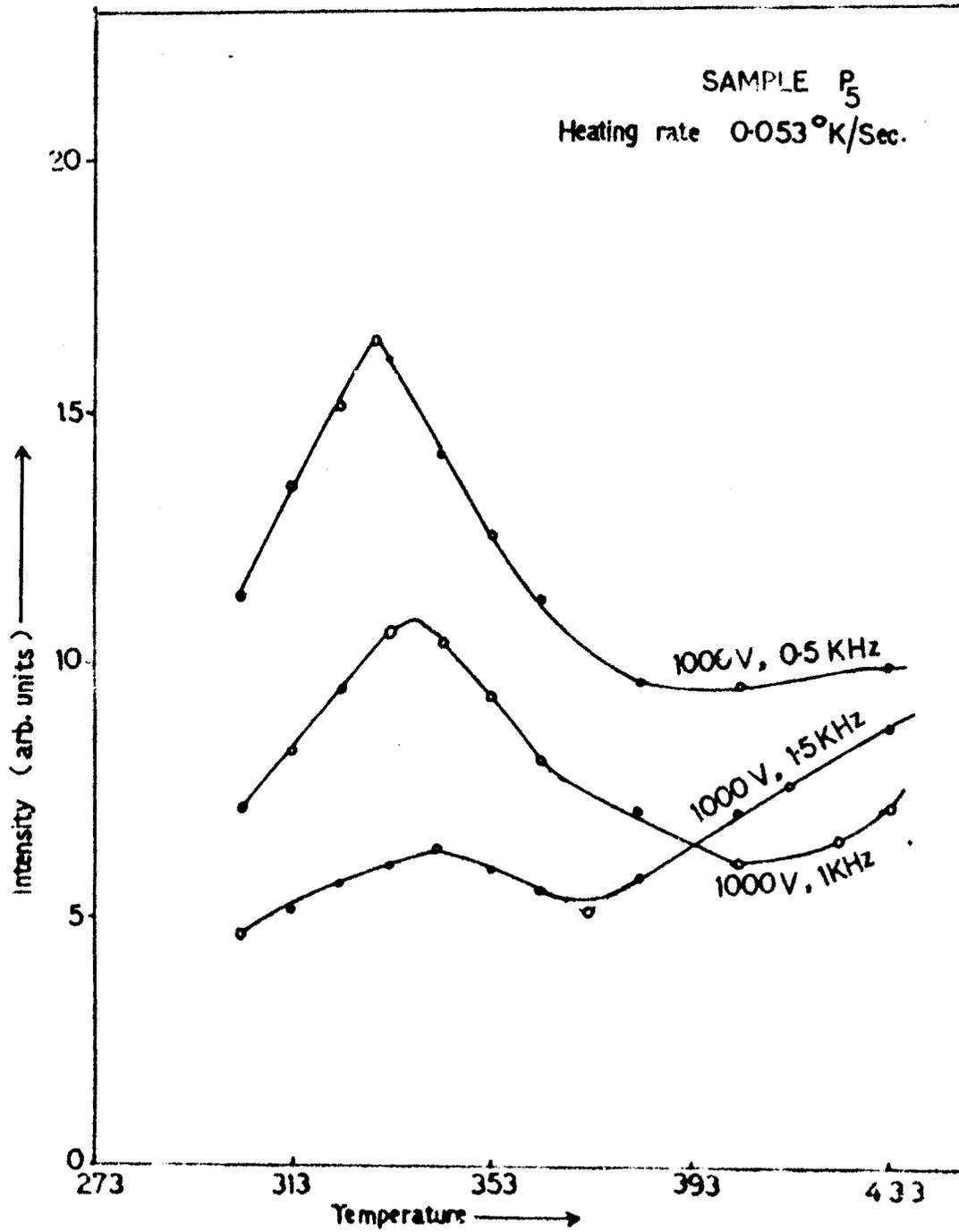
FIG. 45—PLOTS OF INTENSITY V<sub>s</sub> TEMPERATURE AT DIFFERENT FREQUENCIES.
