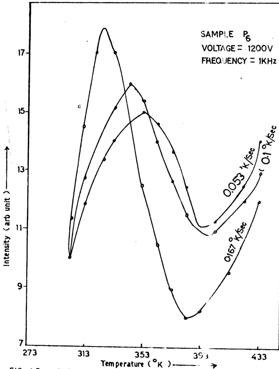
FIG. 4-8—PLOTS OF INTENSITY vs. TEMPERATURE AT DIFFERENT HEATING RATES.
