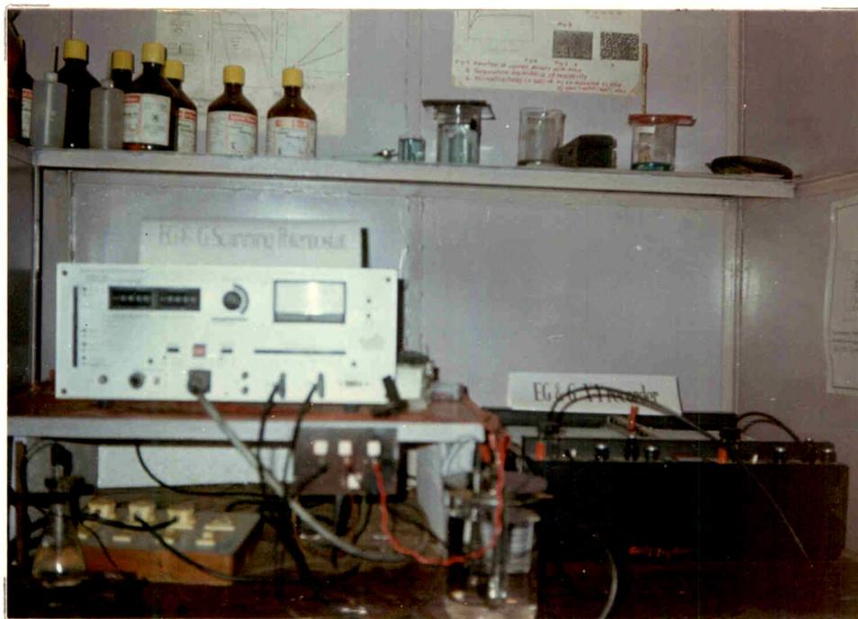
Fig.3.3. Experimental set-up for electrodeposition (photograph).
