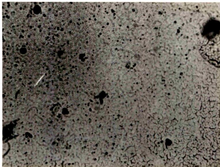
Fig. 8b : Surface Morphology of as deposited titanium
