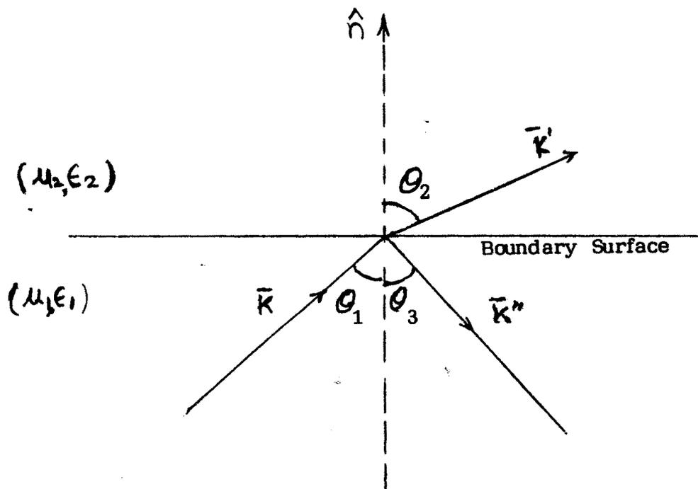
Fig.1.2 : Reflection and Refraction at a Boundary Surface
