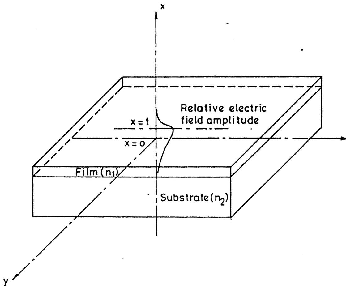
Fig.1.5 : Electric Field Pattern of A Typical  $TE_0$  Guided Wave Mode
