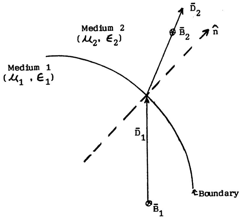
Fig. 1.1 : Propagation of Wave Across A Boundary Surface
