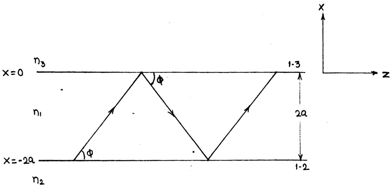
Fig. 1.4 : Propagation of a Ray in Dielectric Slab Waveguide
