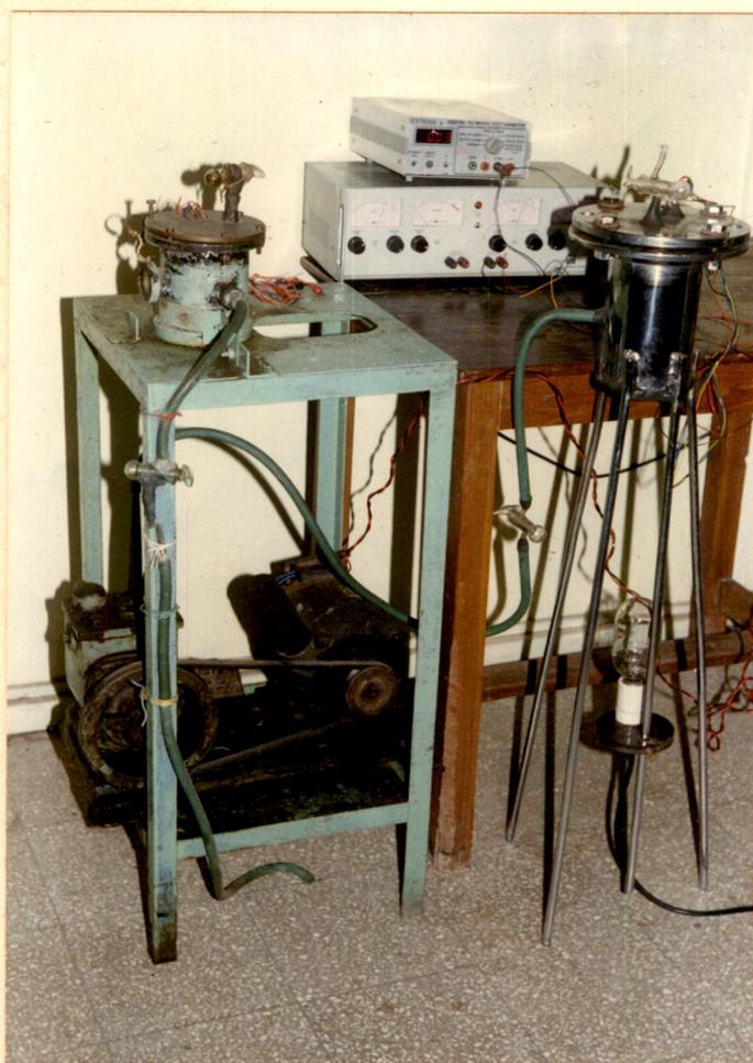
Fig. 3.3 : Photograph of photoconductivity unit.
