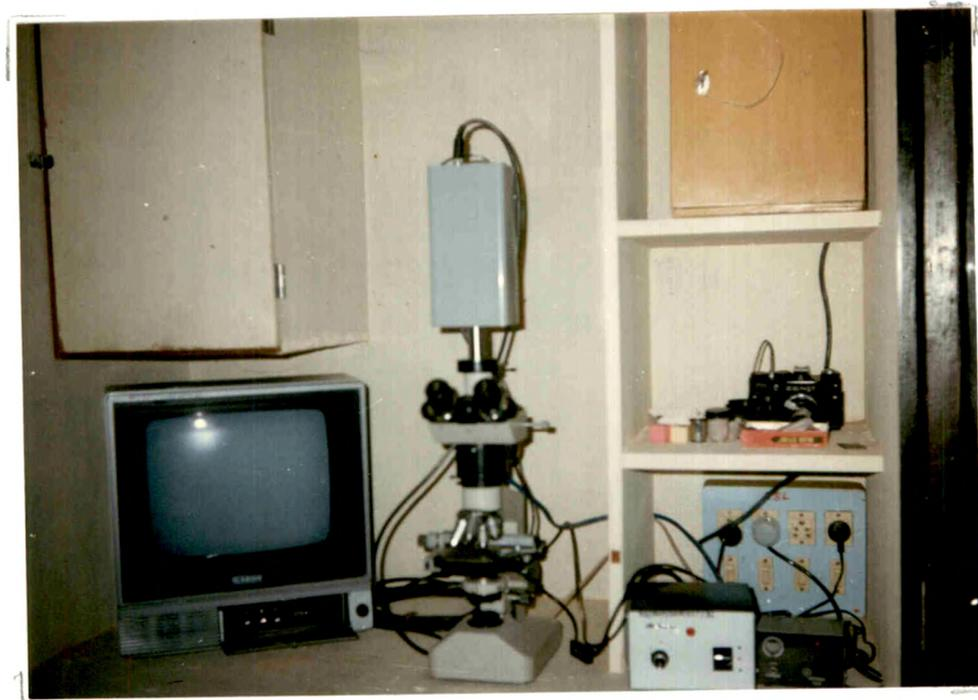
Fig.3.8. Photograph showing set up for microstructure studies.
