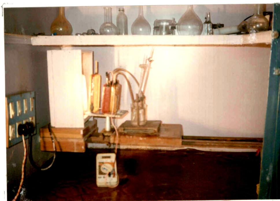
Fig.4.2. Photograph of experimental set up for hydrogen production at static electrolytic condition.
