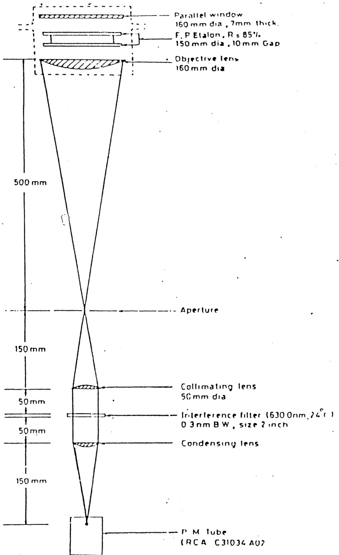
Fig. 4.2. Schematic diagram of Fabry-Perot interferometer (FPI)
