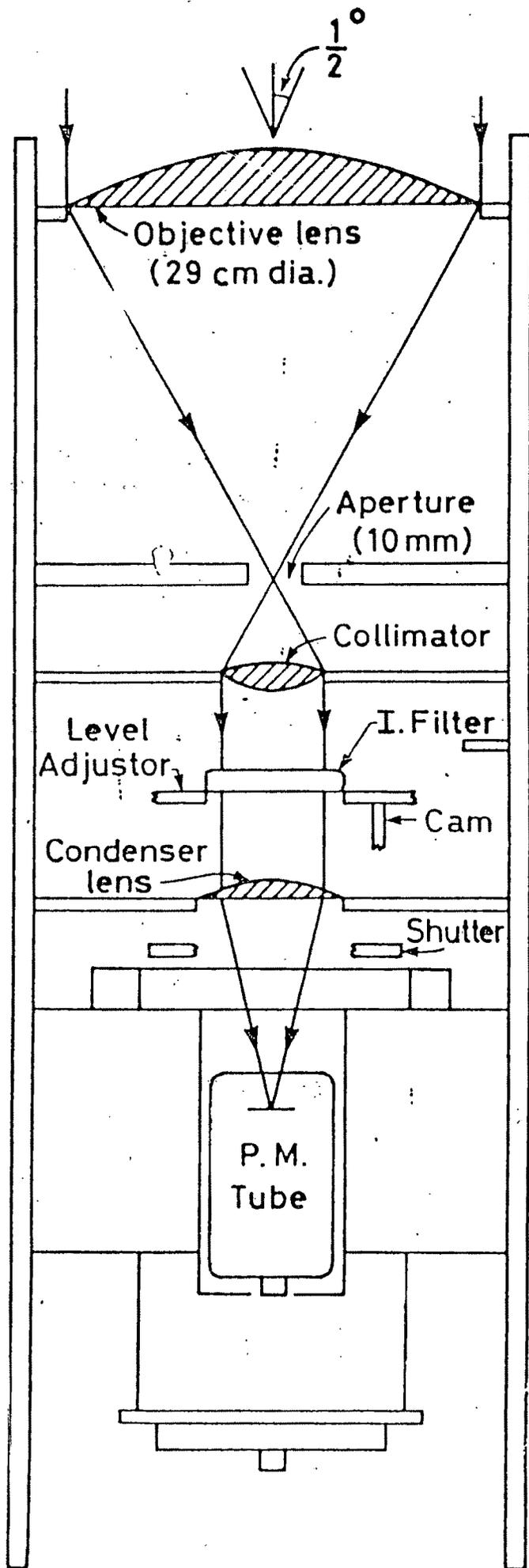
Fig. 4.4 Schematic diagram showing the major parts of tilting photometer.
