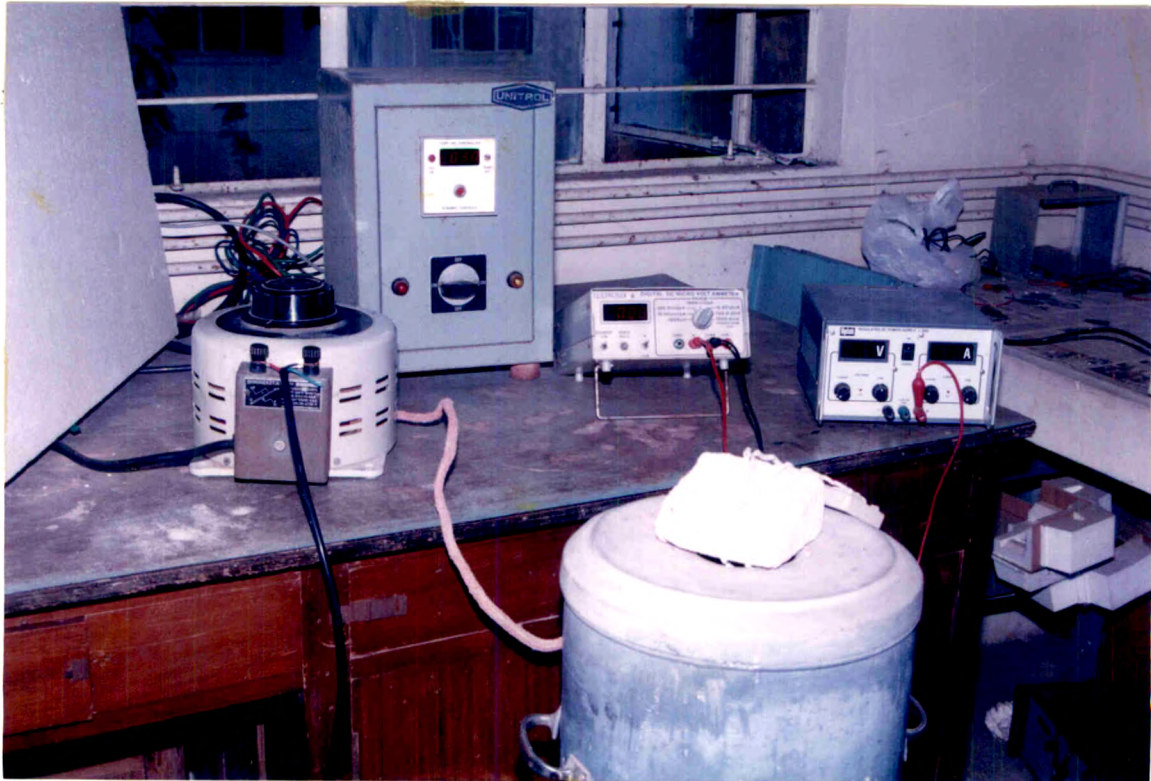
Fig. 3.2: - Experimental set up for the measurement of d.c electric resistivity.
