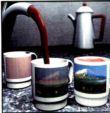
Fig. 1-1. Thermochromic materials change reversibly color when they are heated or cooled.
